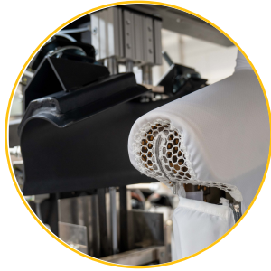
Dispositivo pressa-spalle teflonato (retro) Teflon-coated shoulder pressing device (rear side)
